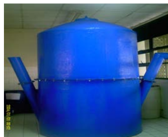
Gambar 3. Reaktor skala 5 m 3 bertipe fixed dome berbahan dasar fiber glass
